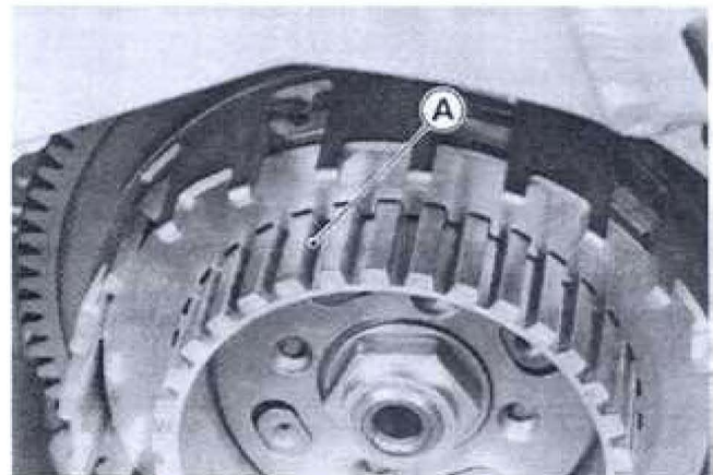
A. Clutch Hub Spline
